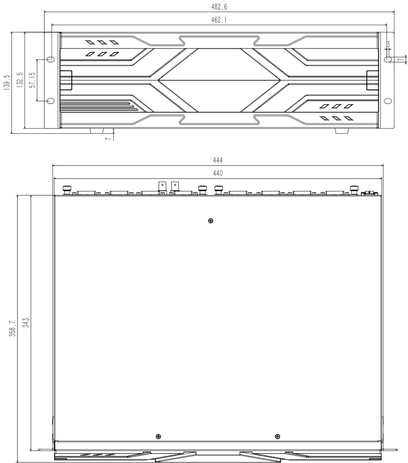
Unit: mm. Linear and angular dimensional tolerances not noted conform to GB/T1804-M.
