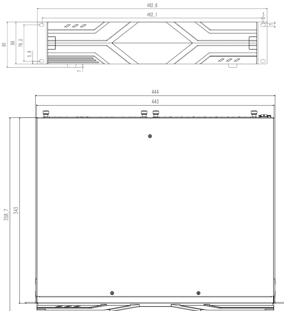
Unit: mm. Linear and angular dimensional tolerances not noted conform to GB/T1804-M.
