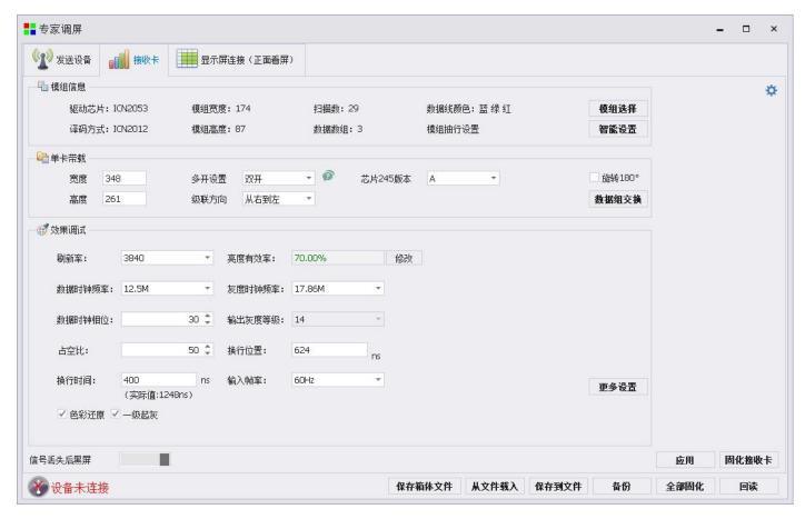
The receiving card interface is used to debug the receiving card parameters, which can be quickly set through module selection, or add module configuration information through smart settings. If there is a previously saved configuration file, it can also be loaded on this page and sent to the receiving card parameter.
