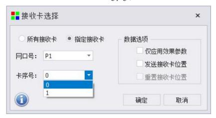
Select all receiving cards or designated receiving cards, the network port number is identified by P1, P2, P3, P4, etc., and the card serial number is identified by 0, 1, 2, 3, etc. 0 identifies all receiving cards of the current network port, 1, 2, 3 represents the specific receiving card serial number of the current network port, and the serial numbers are sorted according to the signal direction. The following picture is the prompt message.
