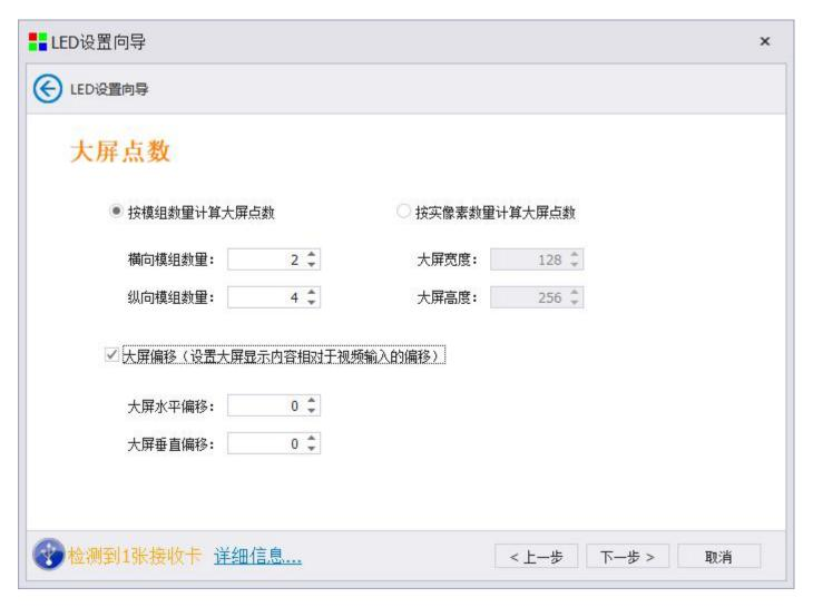
Large screen dots: It can be set according to the number of modules or according to the number of real pixels.
