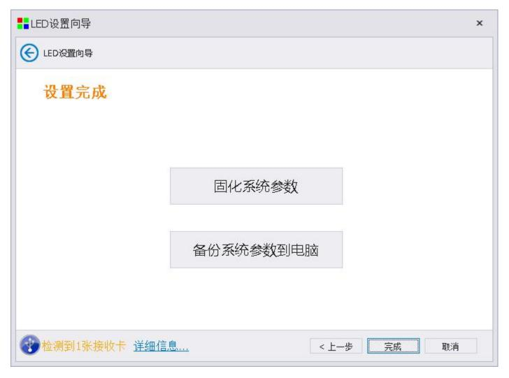
Curing system parameters: curing system parameters to the hardware, and completing the hardware system backup operation, which facilitates the data backup work of one-key repair.
