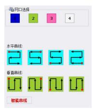
Select the network port number, you can complete the fast string connection of all receiving cards on the screen by selecting the fast string connection method, and you can also use the smart string connection to complete the screen connection.
