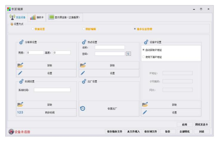
Select Pandora box management: resolution setting; hotspot setting; device IP setting; time setting; factory setting
