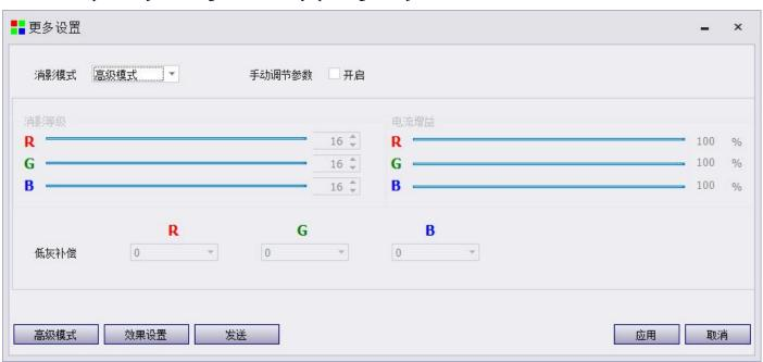
The third step is to click "Effect Settings", select effect settings 1, 2, 3, and 4, and then click "OK" to complete the application of preset effect settings, and select a state where the screen effect is relatively good.
