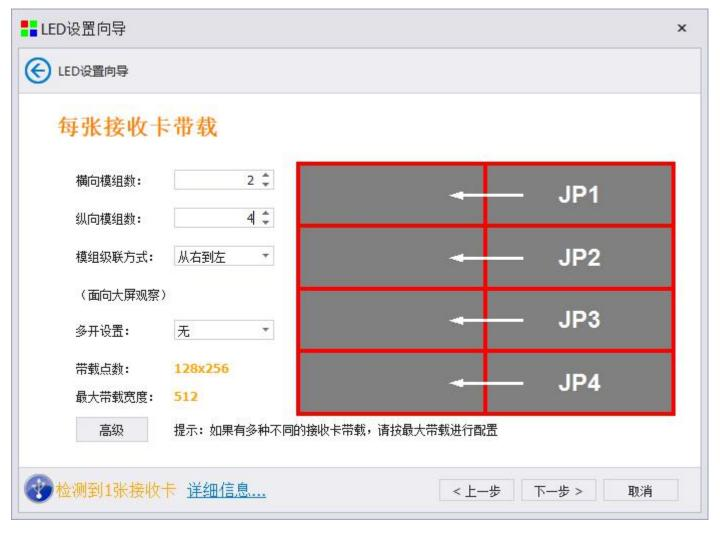
Number of horizontal modules: the number of horizontally loaded modules of a single receiving card
