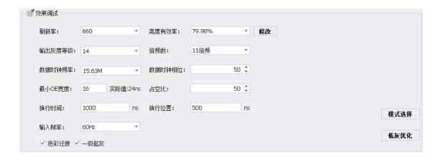
**Mode selection:** The mode selection is used to display the screen effect using the recommended configuration, which is used for dual latch and PWM chips. The first step is to select the chip type.
