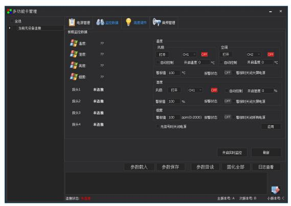
①The monitoring data interface can display the value of environmental variables detected by external probes (light probe, temperature and humidity probe, smoke sensor)
