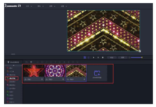
3.2.1 Save plan: After editing the material on the canvas, click Save plan to add it to the plan column, which is convenient for quickly calling this plan again
